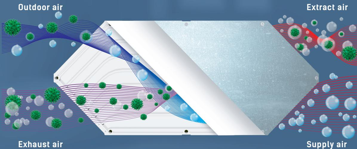
In enthalpy heat exchangers, a vital component known as the vapour-permeable membrane plays a crucial role in optimising performance. Manufactured from a hybrid polymer material, this innovative membrane is carefully engineered to provide exceptional thermal efficiency and moisture transfer capabilities.
