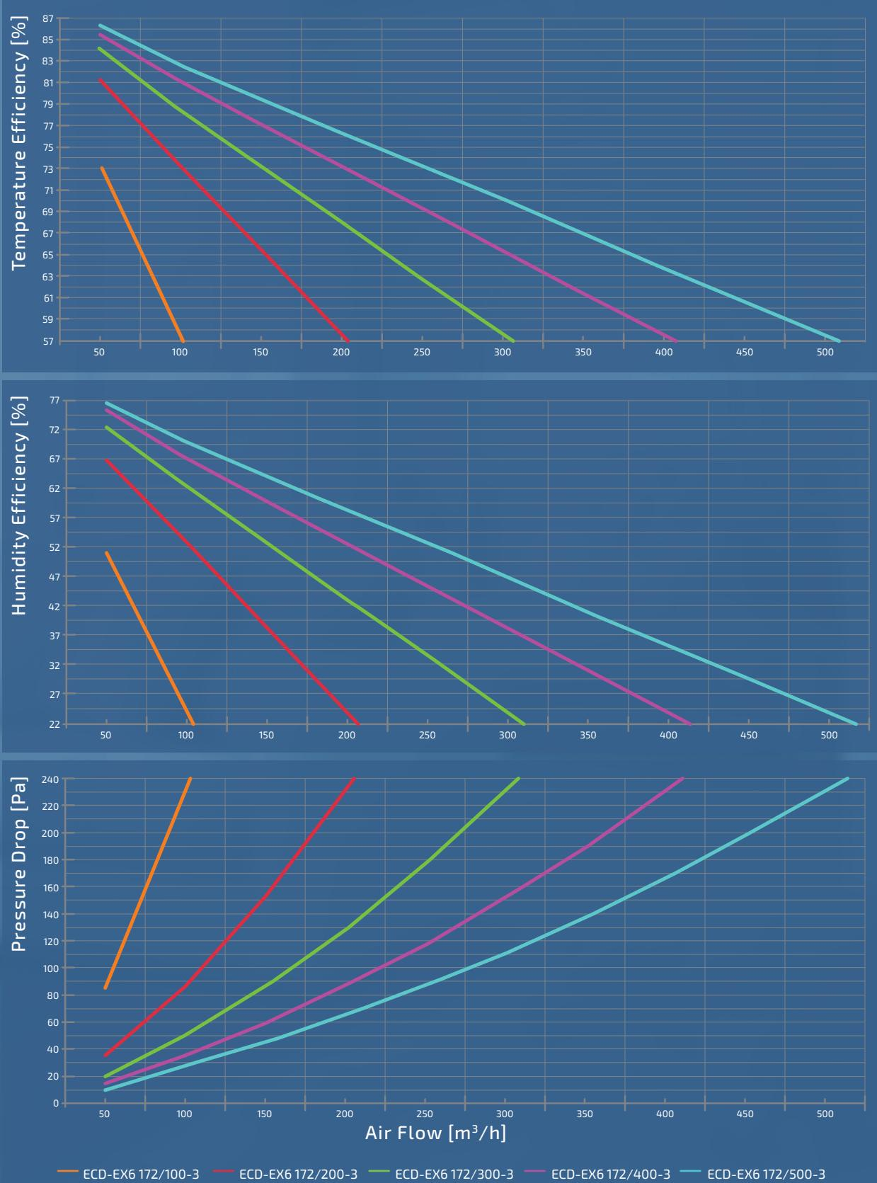
Test results on a ECD-EX6 172/100...500-3 model with a depth of 100...500 mm, test conditions according to DIN EN 13141-7 (as well as EN 308)
