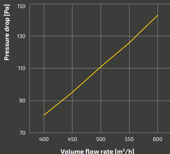
Test results on a HU-312/500-3 model with a depth of 500 mm, test conditions according to DIN EN 13141-7 (as well as EN 308)
