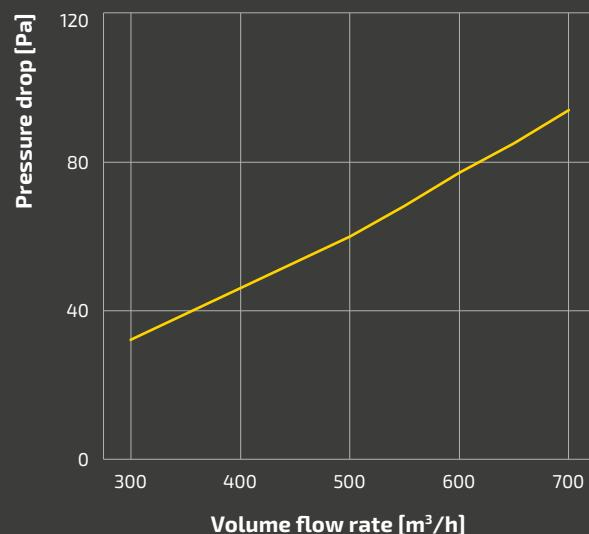
Test results on a HU-477/500-3 model with a depth of 500 mm, test conditions according to DIN EN 13141-7 (as well as EN 308)
