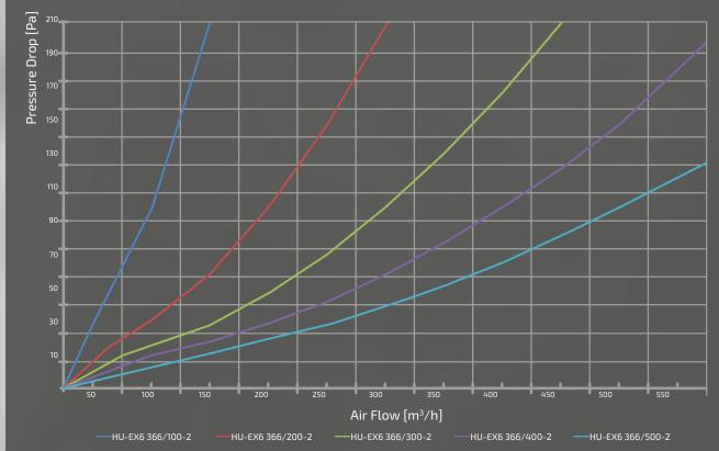
Test results on a HD-EX 366/100...500-2 model with a depth of 100...500 mm, test conditions according to DIN EN 13141-7 (as well as EN 308)
