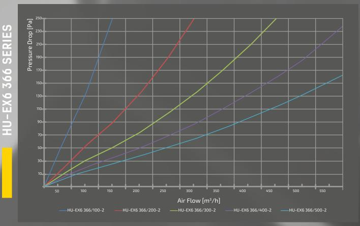
Test results on a HU-EX 366/100...500-2 model with a depth of 100...500 mm, test conditions according to DIN EN 13141-7 (as well as EN 308)
