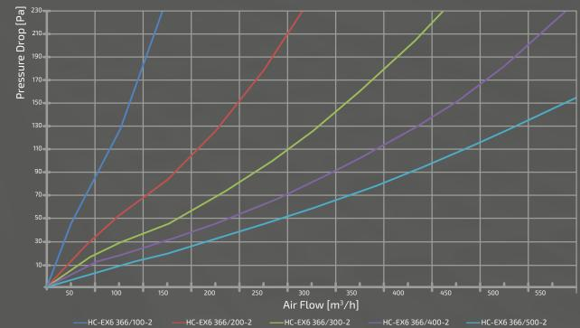
Test results on a HC-EX 366/100...500-2 model with a depth of 100...500 mm, test conditions according to DIN EN 13141-7 (as well as EN 308)
