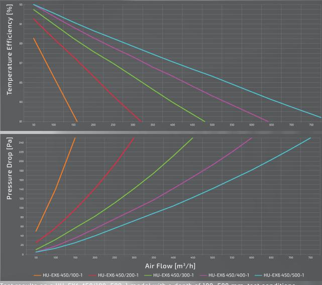
Test results on a HU-EX6 450/100...500-1 model with a depth of 100...500 mm, test conditions according to DIN EN 13141-7 (as well as EN 308)
